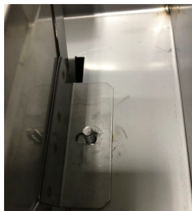
HEARTH BURNER SLOT MUST ENGAGE POST
