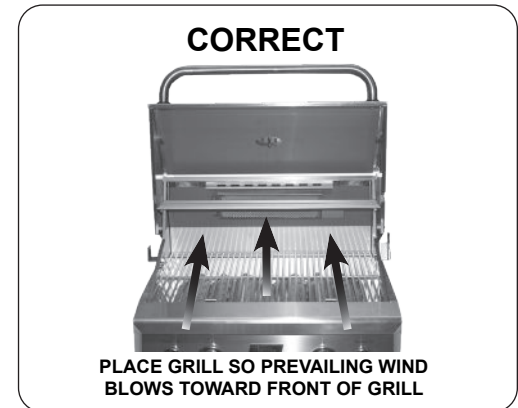
Fig. 13-2 Airflow direction - CORRECT
